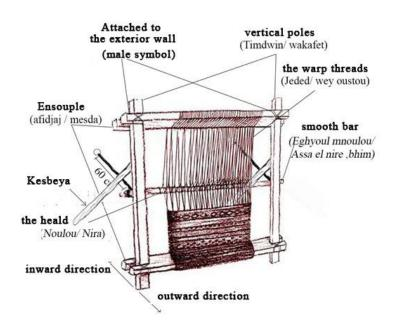
Fig07 : Image of the weaving loom being assembled [Source : Yvonne SAMAMA. Op.cit. p 10]
